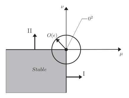
Linear stability diagram for the Van der Pol-Duffing oscillator, undergoing a double-zero bifurcation
