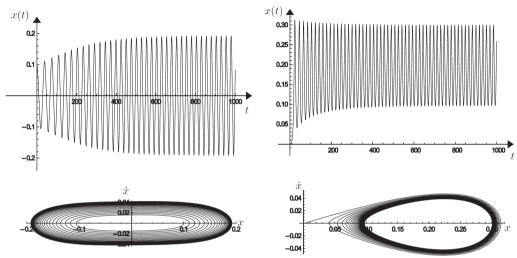
Motions around: (a) a stable *T*-cycle ( $\mu = .01$ ,  $\nu = -.01$ ) and (b) un unstable *B*-cycle ( $\mu = 0.045$ ,  $\nu = 0.01$ ); b = 1,  $c_1 = 2$
