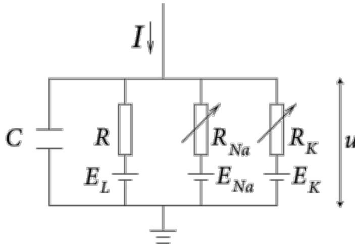
Figure 2.4: Equivalent circuit with  $Na^+$ ,  $K^+$  and leakage channels proposed in Hogkin-Huxley Model. The capacitor representing the membrane potential, Rs for the ionic channels,  $E_i$ s for the Nernst Potential of the  $i^{th}$  ionic specie and I for the external current.
